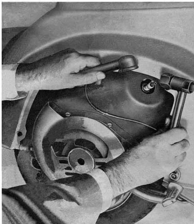
Fig. 10 - Dismantling spark - plug
